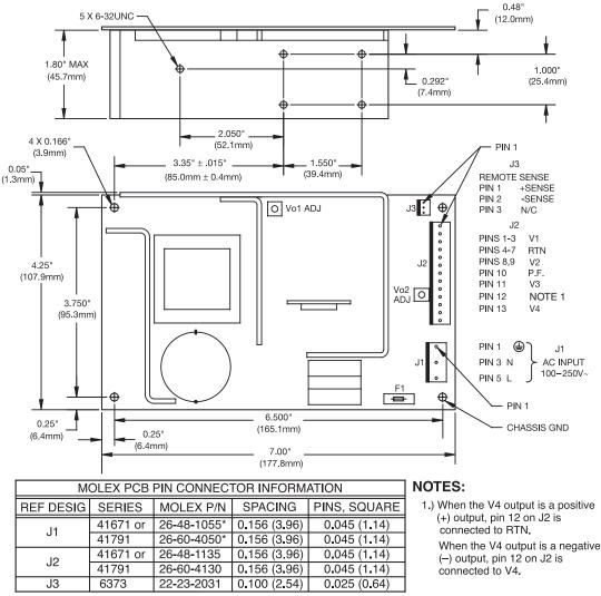
OVERALL SIZE: 7.00" X 4.30" X 1.97" (177.8mm x 109.2mm x 50.0mm) OVERALL WEIGHT: 1.3 lb (0.59 kg)
